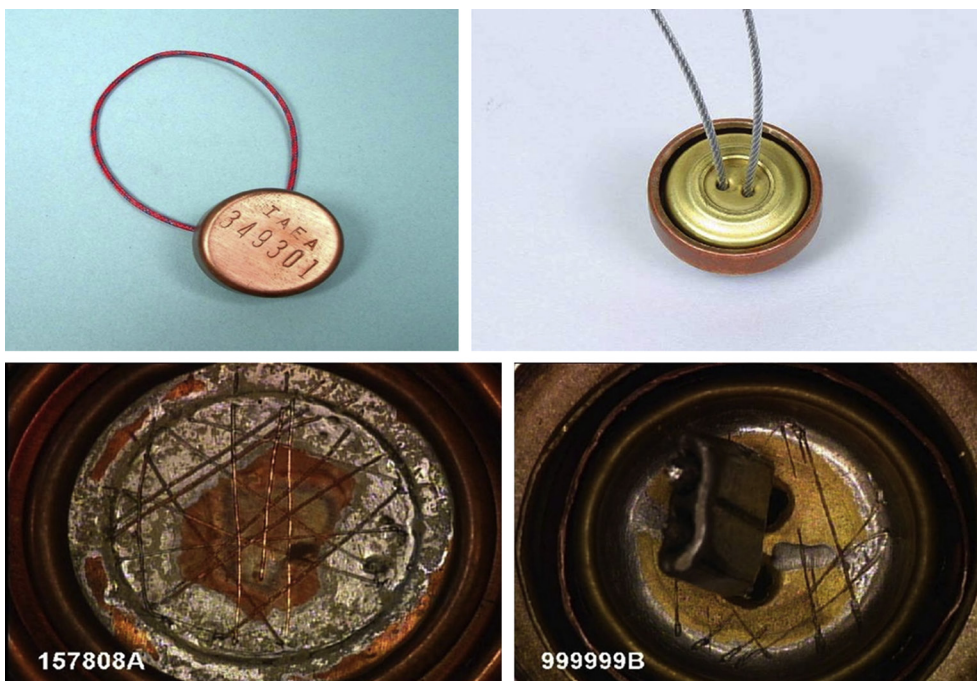
■ FIGURE 7.27 Metal seal. Reproduced with permission from Safeguards Implementation Practices Guide on Facilitating IAEA Verification Activities , IAEA Service Series No. 30.
