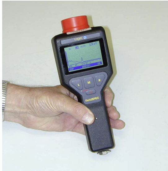
■ FIGURE 7.8 HM-5 Hand Monitor, version five. Reproduced with permission from: International Atomic Energy Agency, Safeguards Techniques and Equipment, International Nuclear Verification Series No. 1 (Rev. 2), IAEA, Vienna (2012).
