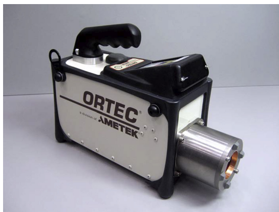
■ FIGURE 7.9 Ortec detective high-purity GE (HPGe). Reproduced with permission from: International Atomic Energy Agency, Safeguards Techniques and Equipment, International Nuclear Verification Series No. 1 (Rev. 2), IAEA, Vienna (2012).
