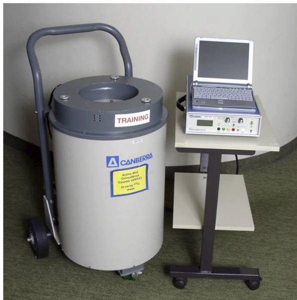
■ FIGURE 7.12 (A) High-level neutron coincidence counter; (B) active well neutron coincidence counter.
