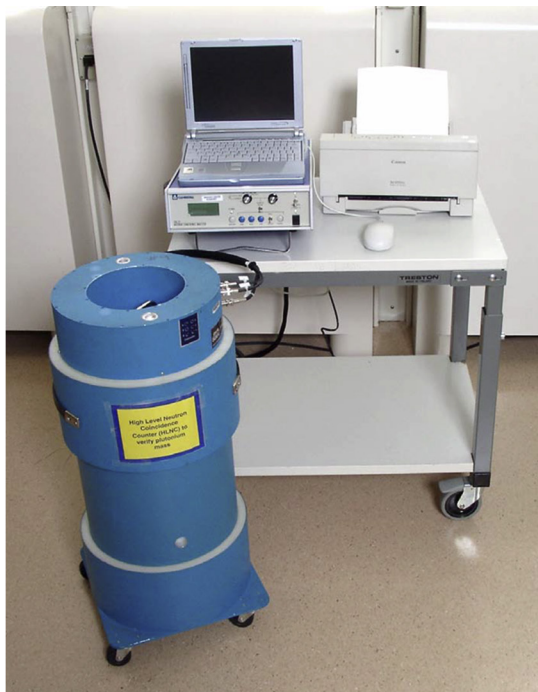
■ FIGURE 7.12 (A) High-level neutron coincidence counter; (B) active well neutron coincidence counter.
