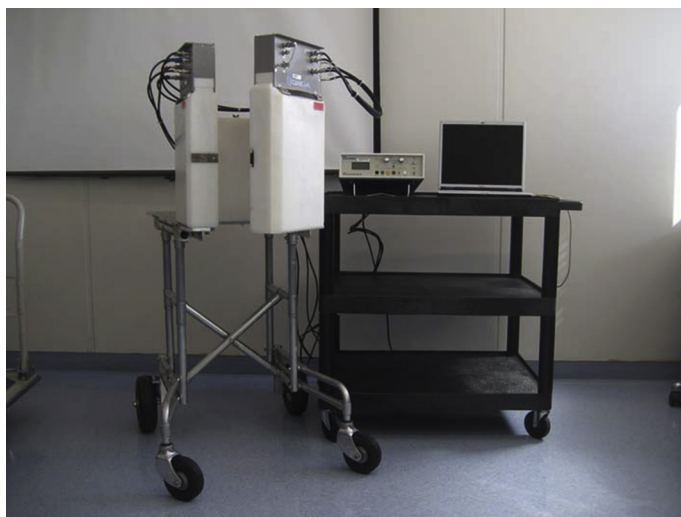
■ FIGURE 7.13 Uranium neutron coincidence collar. Reproduced with permission from: International Atomic Energy Agency, Safeguards Techniques and Equipment, International Nuclear Verification Series No. 1 (Rev. 2), IAEA, Vienna (2012).
